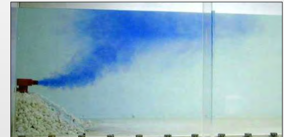
Hot Water Diffusion Analysis by Model test
